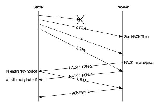
Figure 17 Elimination of Retransmission using Hold-off Timer
