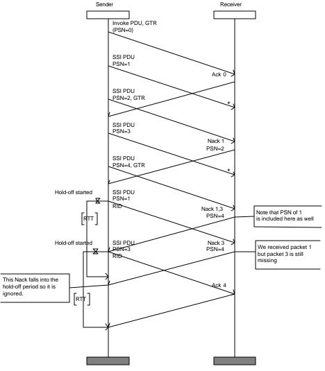
Figure 18 Filtering of Nacks during Hold-off Period
