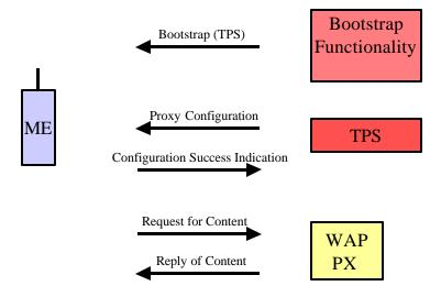
Fig. 3 - Logical model showing the three typical steps needed to get access to content. The device is bootstrapped with information about a TPS. The TPS then loads the mobile equipment with information about access points and proxies. As a result the device is able to access content via one or more WAP proxies.
