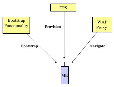
Fig. 5 - The provisioning framework deals with two concepts, the bootstrap and the continuous provisioning. The gateway navigation mechanism is also closely related. Each of these are logically linked with each other through common content.
