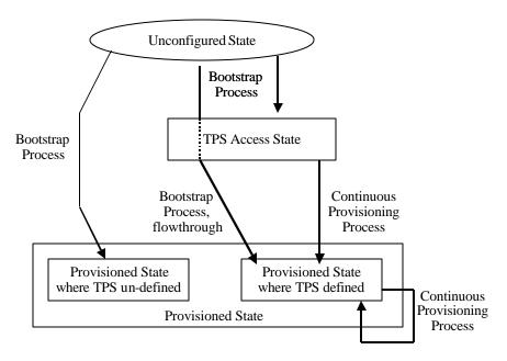
Fig. 2 - The configuration context normally is in the provisioned state. The two boxes for the provisioned state show that it is possible to do continuous provisioning only if a Trusted Proxy and a Provisioning URL is defined, i.e. the TPS access state has been visited in the bootstrap.
