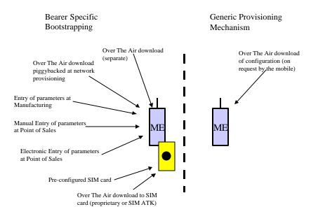
Fig. 4 - The separation between the bearer specific bootstrapping and the generic provisioning. The bootstrapping process can be adapted to the bearer network type, while the continuous provisioning (updates) is based on mostly generic concepts.
