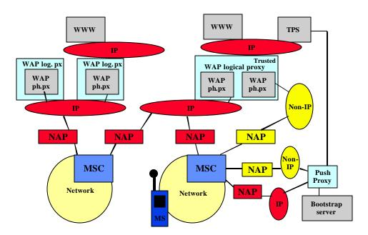
Fig. 1 - The provisioning process is used to provide the mobile device with an abstraction of the network topology, and the addresses and methods to access particular resources. The picture shows a typical structure with WAP proxies and Network Access Points (often a Remote Access Server) needed to reach a particular proxy.
