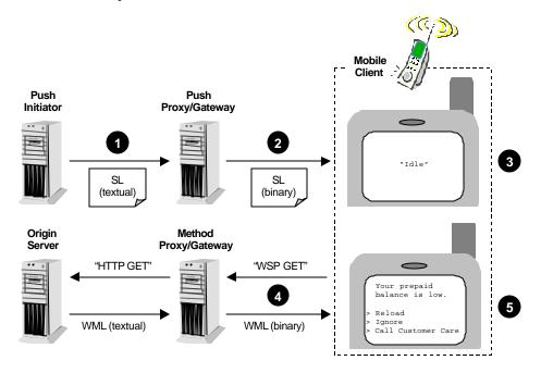
Figure 1: Service Loading - the basic concept
