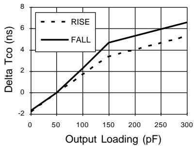
**GAL16V8C-5/-7: TYPICAL AC AND DC CHARACTERISTIC DIAGRAMS**
