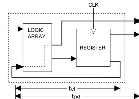
**f<sub>max</sub> with Internal Feedback 1/(tsu+tcf)**
