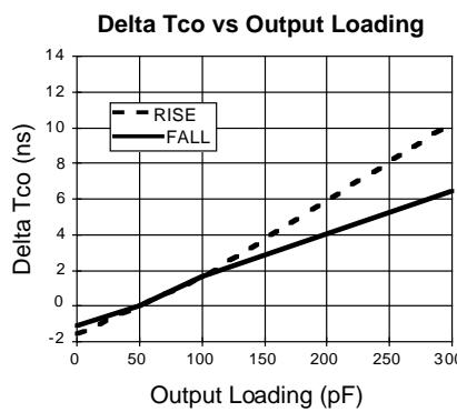
**GAL16V8D-3: TYPICAL AC AND DC CHARACTERISTIC DIAGRAMS**
