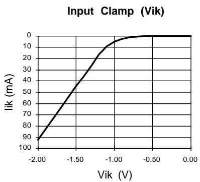
**GAL 16V8B-15/-25: TYPICAL AC AND DC CHARACTERISTIC DIAGRAMS**
