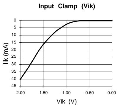
**GAL16V8B-7/10: TYPICAL AC AND DC CHARACTERISTIC DIAGRAMS**
