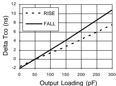
**GAL16V8B-15/-25: TYPICAL AC AND DC CHARACTERISTIC DIAGRAMS**
